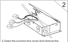
2.Open the junction box cover and remove the appropriate knockout(s) on the side panel. Insert the electrical supply cable through the knockout and secure with a cable connector (sold separately). Using quick-connect push-in terminals, connect the ground wire to the green wire terminal; black wire to black wire terminal; white wire to white wire terminal.
