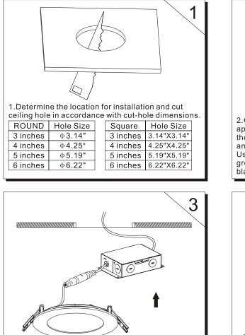
3.Place all wiring and connections back in to the box and close the cover. Connect the driver to the light panel.Insert junction box through the mounting hole.
