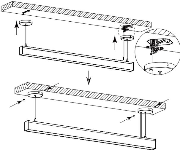
Thread the power cable (provided) through the canopy with power feed hole and wiring in the J box (not provided), Black=L, White=N, Green or Yellow/Green=C, Purple=Dim+, Pink=Dim-. After the wiring is done, use M4x8 screws to fix two canopies to the crossbars.
