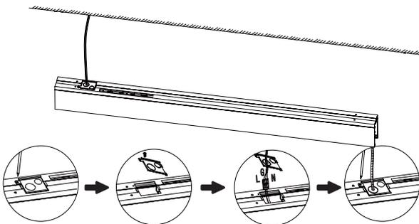
Open the back lit cover on the fixture by unscrew the screw, take out the AC power cord and make wiring connection, Black=Line, White=Neutral, Yellow/Green=G, Purple=Dim+, Pink=Dim-. Then lock the back lit cover with screw.
