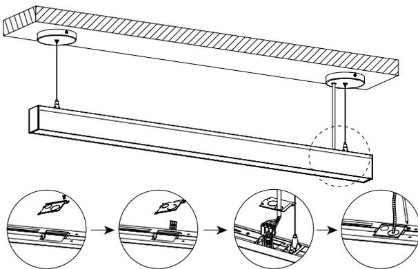
Open the back cover on the fixture and take out the terminal block, thread another end of the power cable to the outlet of the back cover to make wiring, plug white wire into terminal N, black wire into terminal L and green wire into grounding terminal, pink and purple wire are for dimming purpose, leave them alone if not use dimming. After the wiring is done, attach the back cover to the fixture.
