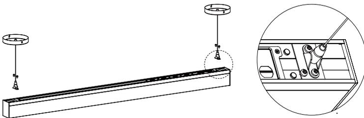
Use M5 x 6 screws to attach the suspension cables to the two movable brackets of the fixture.
