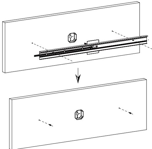
Drill mounting holes on the wall based on the distance on wall bracket, then put plastic anchor into the mounting holes.
