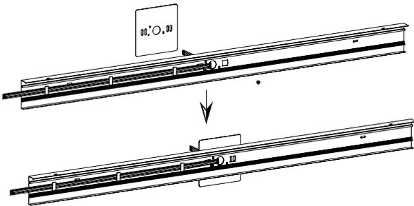
Attach cover plate to wall mount bracket by using M4x8 screw
