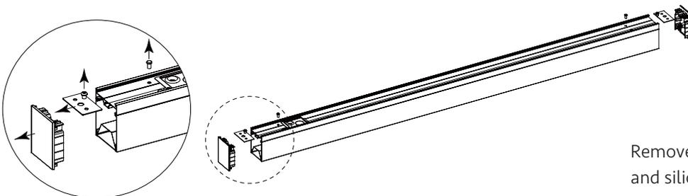
Remove both ends caps, two suspension brackets and silicone plugs from the luminaire.
