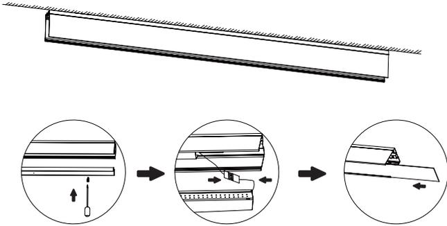
After the fixture is fixed, follow the steps in sequence, screw the LED module to the housing, connect the fast connectors between the PCB and LED driver, then slide the PC cover into the housing.
