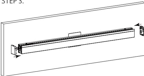
Tuck wires into the luminaire, and place wall mount end caps onto both ends.
