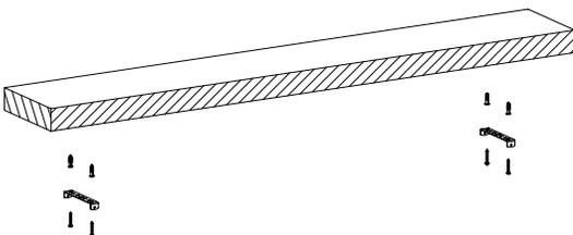
Use anchors and self-tapping screws to fix the two crossbars on the mounting surface.
