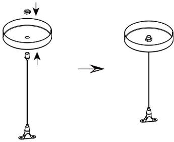
Take out the two canopies, insert the suspension cables in and fasten them with M9 nuts.
