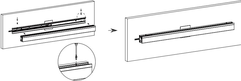
Attach luminaire to wall mount bracket by using two M5 x12 screws.
