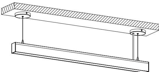
Adjust the height of the fixture by press the button on the gripper, pull or push the cable carefully to raise or lower the fixture. Then turn on the electricity to verify your successful installation.
