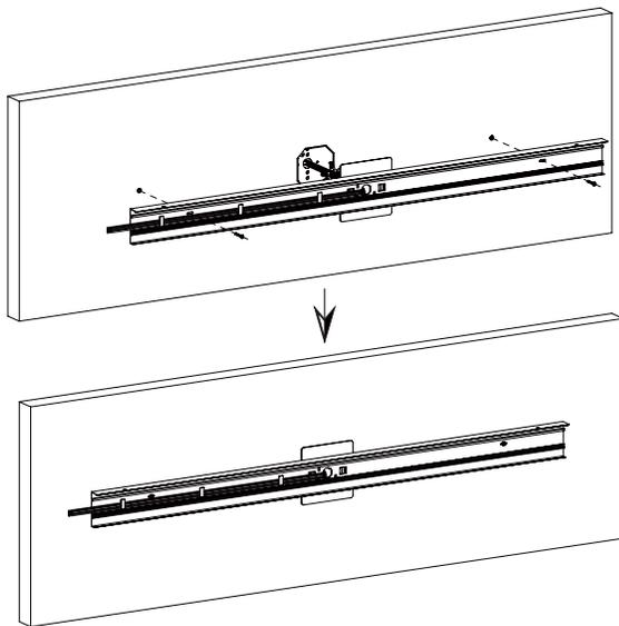
Feed power cord through cover plate and use wire nuts to connect wires in the J-box (not provided).
