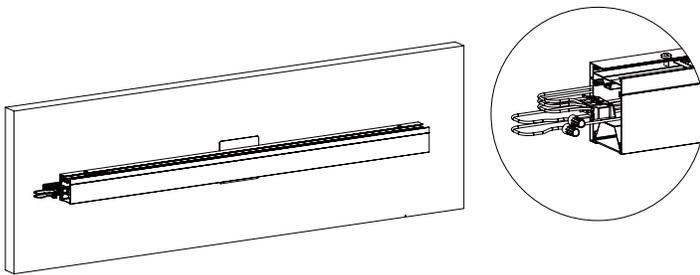
Connect power cord to luminaire's input wires and plug N,L,G wires into the terminal block.
